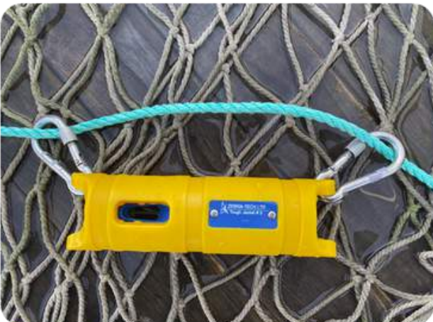
Example of Tough Jacket #3 rope attachment method
