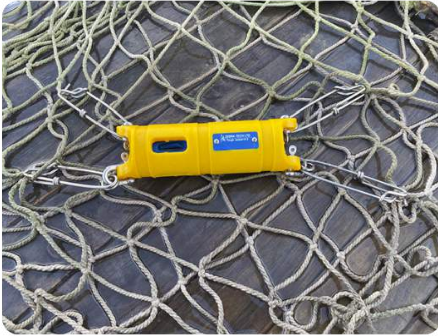
Net attachment example with Tough Jacket #3
