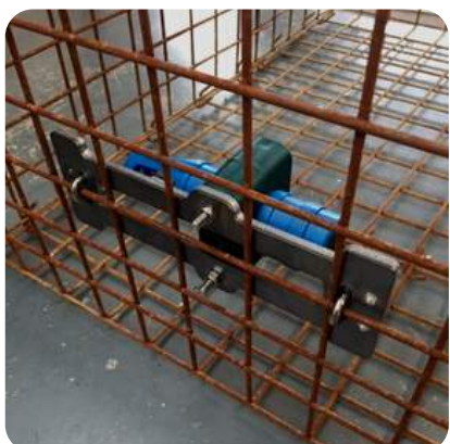
Mounting Plate #2 with Stauff Clamp
