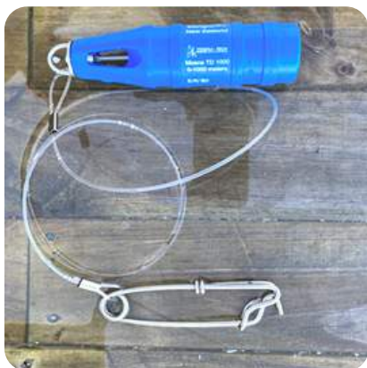
Tow ring attachment for long lining
